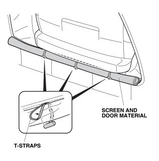
6. Stretch the bottom elastic strap across the rear face of the bumper. Make sure the tent material is tight against the rear face of the bumper, with the exhaust pipe outside the tent. Go outside of the tent, and visually inspect the location of the exhaust pipe to verify its location.
