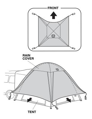
12. Attach the hook on each corner of the rain cover to the tent ring on the tent. Wrap the Velcro tabs around each pole to hold the rain cover in place.
