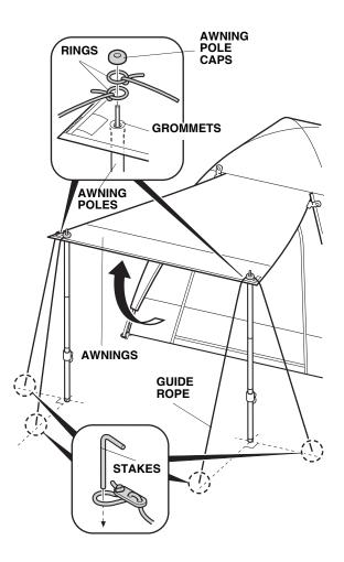
15. Pull the awning tight, adjust the height of the awning using the telescopic pole, and secure the awning to the ground using an additional stake and guide rope. Secure the other pole using the same procedure. If necessary, adjust the guide rope length using the adjuster on the rope.
