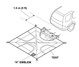
Unfold the tent poles (11 sections each) and assemble the connected sections into one long pole. Assemble the other tent pole the same way.
