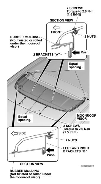
14. Tighten the two screws and two nuts on the front of the vehicle first, then tighten the two screws and two nuts on each side.
