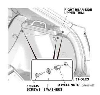
20. Place a washer onto the snap-screw and install three snap-screws.
