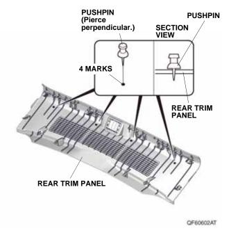
7. While wearing eye protection, drill the four pierced marks with a 3 mm drill bit, with a 6 mm drill bit, then finish with an 8 mm drill bit.
