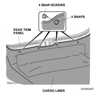
35. Lay down the cargo liner on the rear seat-backs and attach the fasteners to the rear seat-backs as shown.
