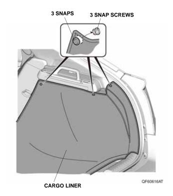
30. Secure the fasteners to the right rear side lower trim as shown.
