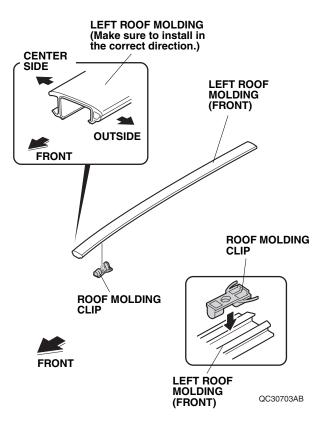
Install the roof molding left cover.
