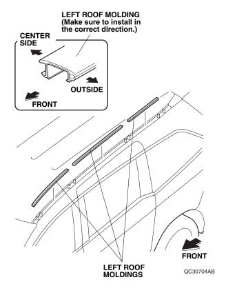
Install the left side roof rail with six Torx nuts. Make sure the roof rail is installed in the correct position. Torque the Torx nuts to: 10 N·m (7.3 lb·ft)
