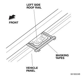
17. Hook the left center roof rail cover to the left side roof rail as shown.
