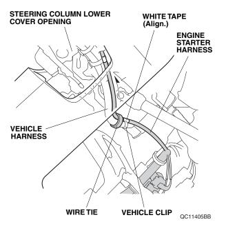
22. Align the white tape on the engine starter harness with the vehicle clip, and secure the engine starter harness to the vehicle harness with one wire tie as shown.
