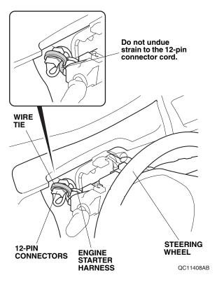
30. Install the harness cover, and re-plug the cable reel 20-pin connector unplugged in step 26.
