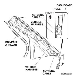
56. Route the antenna cable along the vehicle harness, and secure it to the vehicle harness with one wire tie.
