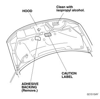
69. Remove the adhesive backing from the caution label, and attach the caution label to the hood in the area shown.
