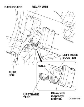
38. Unplug the vehicle 2-pin connector from the relay unit, and plug it into the engine starter harness 2-pin connector. Plug the remaining engine starter harness 2-pin connector into the relay unit.
