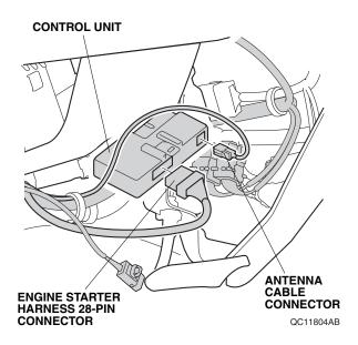
Install the control unit to the control unit bracket.
