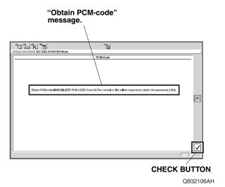
Input the PCM-code, then click the check button. NOTE: To ensure security, the PCM-code (password) is changed everyday, so it is impossible to register the remote control engine starter if the dates of the PCM-code acquisition and registration are different. The date of the HDS/MVCI tester should also be the same.
