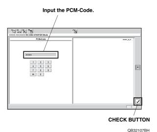
10. The following message will display: The registration of the Remote Control Engine Starter Unit has been completed. Turn the ignition switch off.
