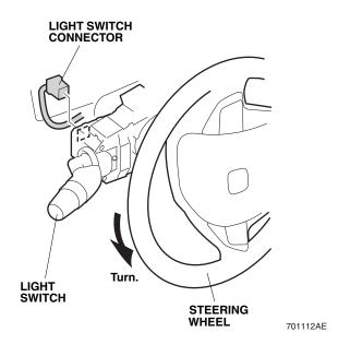
38. Remove two self-tapping screws from the light switch. While pushing the retaining tab, slide the light switch, and remove it from the steering column. Do not pull on the lever when removing the case. NOTE: Do not damage the tab hole on the steering column.
