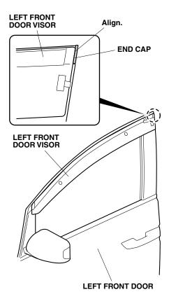
While applying light pressure against the left front door visor, carefully remove the adhesive backings. Push up on the front brackets while removing the adhesive backings.
