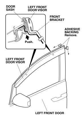
10. Using the palm of your hand, firmly press the left front door visor against the door sash.
