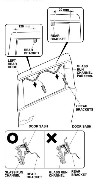
13. Install the glass run channel to secure the two rear brackets. Be sure the brackets are installed tightly to the door sash, and that the glass run channel is properly seated.
