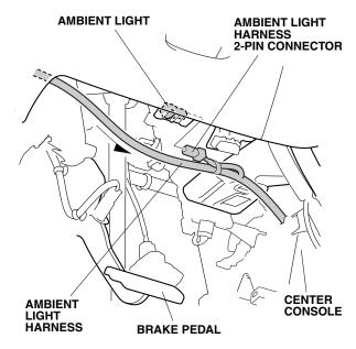
11. Plug the ambient light harness 2-pin connector into the ambient light.
