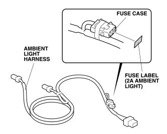
7. Plug the ambient light harness 12-pin connector into the driver's fuse box.
