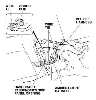
15. Route the ambient light harness along the vehicle harness, and to the blower motor. Secure the ambient light harness to the vehicle harness with two wire ties. Secure the wire tie next to the vehicle clip.
