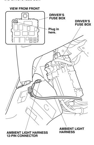
8. Secure the ambient light harness to the vehicle harness with one wire tie.
