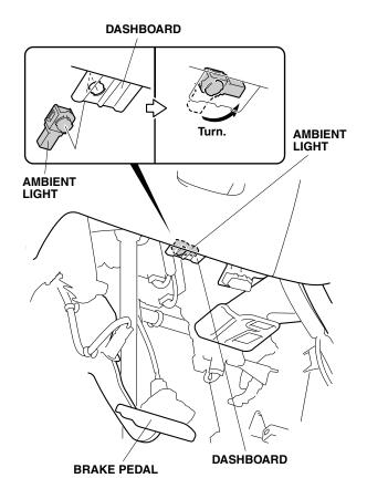
10. Route the ambient light harness to the center console as shown.
