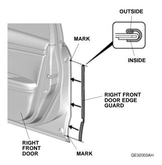
Starting at the character line, tap the right front door edge guard into position with a series of light taps using a rubber mallet, then work up and down. Make sure the position of the right front door edge guard is correct.
