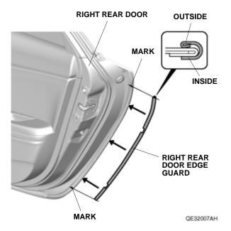
15. Starting below the character line, tap the right rear door edge guard into position with a series of light taps using a rubber mallet, then work up and down. Make sure the position of the right rear door edge guard is correct.
