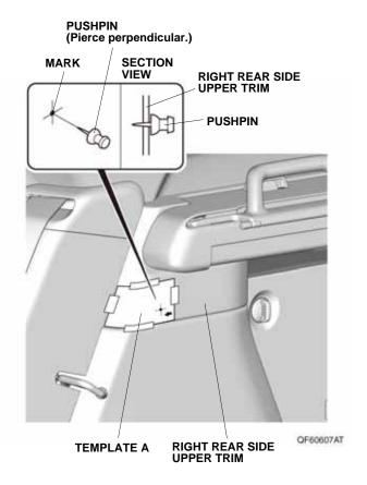
15. Using a pushpin, pierce the right rear side upper trim through the templates at the two locations shown on the templates.
