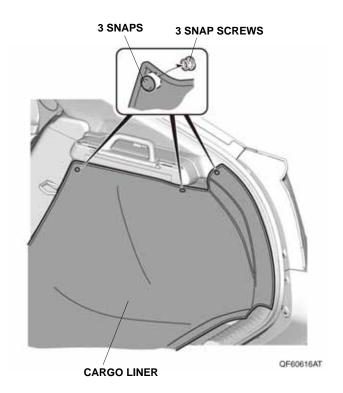
30. Secure the fasteners to the right rear side lower trim as shown.
