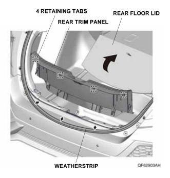
4. Using a felt-tip pen, mark the rear trim panel as shown.
