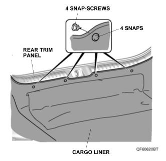
35. Lay down the cargo liner on the rear seat-backs and attach the fasteners to the rear seat-backs as shown.
