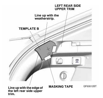
23. Using a pushpin, pierce the left rear side upper trim through the templates at the two locations shown on the templates.
