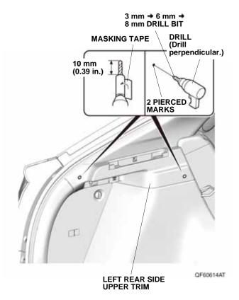
26. Using a file, remove any burrs from the holes.
