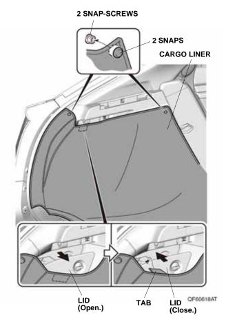
32. Open the lid and put the tab in between the lid and the left rear side lower trim. Close the lid.
