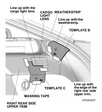
14. Using a pushpin, pierce the right rear side upper trim through the template at the location shown on the template.
