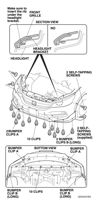
14. Secure the left and right front under spoilers to the front bumper with two bumper clips A, two bumper clips B (long), and two self-tapping screws.
