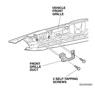
7. Install the front grille duct to the front grille with the two self-tapping screws removed in step 6.
