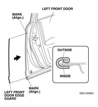
8. Starting at the feature line, use a rubber mallet to tap the left front door edge guard into position with a series of light taps, then work up and down. Make sure the position of the left front door edge guard is correct. Once in place, do not attempt to remove, reposition, or reinstall the left front door edge guard.
