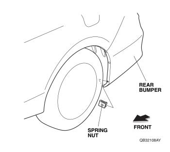
13. Install the left rear splash guard to the rear bumper with two washer-screws and the screw removed in step 7. Install them in this order 1→2→3. Make sure there is no gap between the left rear splash guard and the vehicle body. If there is a gap, loosen the two washer-screws and one screw, hold the splash guard against the body, and tighten the two washer-screws and one screw.
