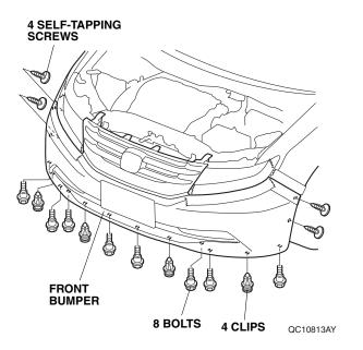
• On each side, release eight retaining tabs from the front bumper.
