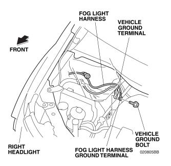
14. Locate the 1-pin connector blue-taped to the vehicle harness. Remove the blue-tape to release the 1-pin connector.
