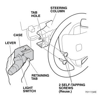
39. Install the new light switch to the steering column with two self-tapping screws removed in step 38. NOTE: Do not push on the lever when installing the case. Push in on the case and set the retaining tab into the tab hole.
