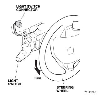
38. Remove two self-tapping screws from the light switch. While pushing the retaining tab, slide the light switch, and remove it from the steering column. Do not pull on the lever when removing the case. NOTE: Do not damage the tab hole on the steering column.
