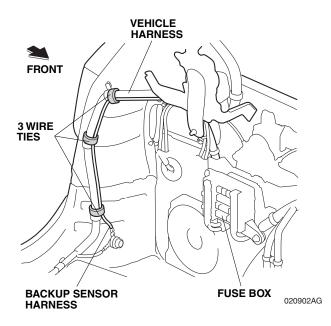
45. Route the backup sensor harness 2-pin connector along the vehicle harness.
