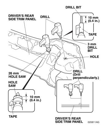
30. From inside of the driver's rear side trim panel, wear an eye protection and drill one hole with a 3 mm drill bit.
