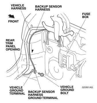
43. Remove one vehicle ground bolt and secure the backup sensor harness ground terminal to the vehicle ground terminal with the vehicle ground bolt just removed.
