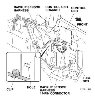
59. Secure the clip on the backup sensor harness to the hole on the control unit bracket as shown.
