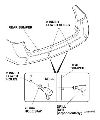
Insert the right center sensor (Blue) and left center sensor (Blue) to the rear bumper. NOTE: The left center sensor (Blue) has the yellow dot label.
