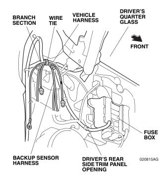
42. Route the backup sensor harness ground terminal along the vehicle harness.
