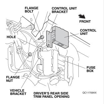
Route the backup sensor harness 14-pin connector, 58. and plug it to the control unit.
