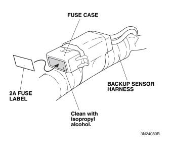
41. Secure the backup sensor harness to the vehicle harness with one wire tie as shown.
