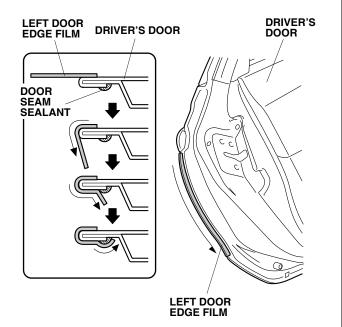
8. Using a shop towel, wipe the excess 3M protective tape application solution from the left door edge film. NOTE: Allow the left door edge film to dry thoroughly.
