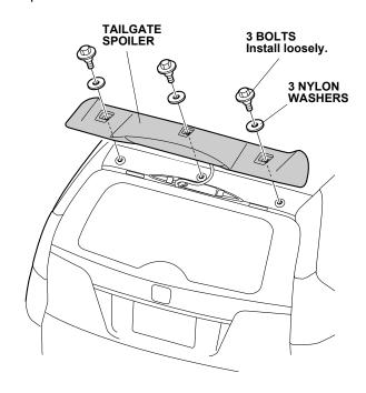
41. Use the palm of your hand to firmly press the tailgate spoiler to the tailgate. Make sure the hook and loop fasteners are secure.
