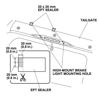
23. Attach one 20 x 20 mm piece of EPT sealer over each high-mount brake light mounting hole.
