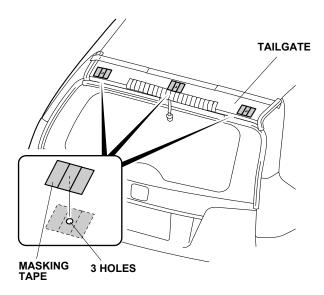
15. While wearing eye protection, use an 11 mm hole saw to enlarge the three holes in the tailgate.
