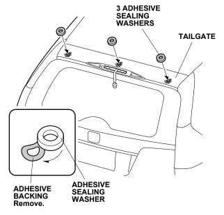
20. Remove the adhesive backing from each adhesive sealing washer, and attach one washer over each jack nut.
