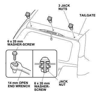
19. Using isopropyl alcohol on a shop towel, clean the tailgate where the three adhesive sealing washers will attach.
