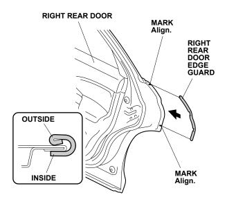
14. Starting at the feature line, tap the right rear door edge guard into position with a series of light taps using a rubber mallet, then work up and down. Make sure the position of the right rear door edge guard is correct. Once in place, do not remove, reposition, or reinstall the right rear door edge guard.
