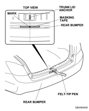
3. Align the rear bumper applique with the rear bumper and check the rear bumper applique position. Remove the rear bumper applique.
