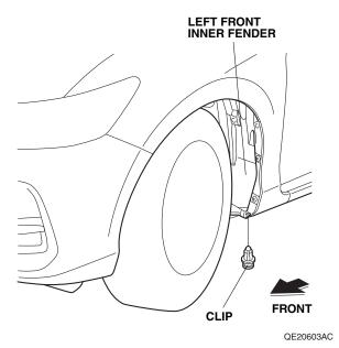
4. Install the left front splash guard to the left front inner fender with two washer-screws and the clip removed in step 3. Install them in this order 1→2→3. Make sure there is no gap between the left front splash guard and the vehicle body. If there is a gap, loosen the two washer-screws, hold the splash guard against the body, and tighten the two washer-screws.
