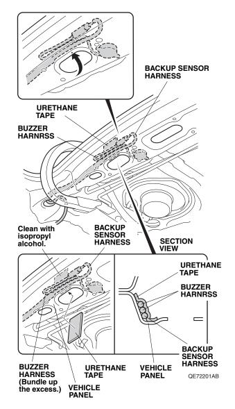
25. Bundle up the excess buzzer harness, and secure the buzzer harness and backup sensor harness to the vehicle panel with one urethane tape as shown.
