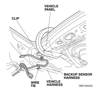
22. Secure the backup sensor harness to the vehicle harness with one wire tie.
