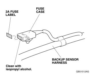
20. Secure the backup sensor harness to the vehicle harness with one wire tie.
