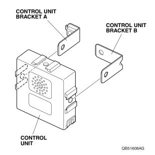
32. Secure the control unit to the vehicle panel with the flange bolt at the location shown.
