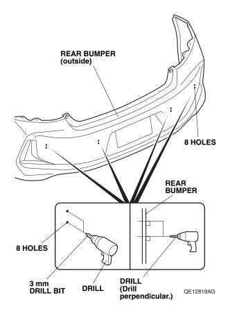
• Using a 24 mm hole saw, enlarge the outboard (left and right corner sensor) bumper holes by drilling the lower 3 mm holes. Remove any burrs.
