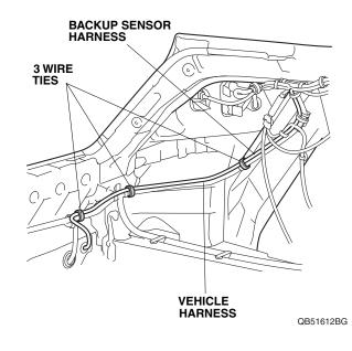
39. If equipped with vehicle another harness, install the wire tie with holder to the backup sensor harness8-pin connector, and secure it to the vehicle harness.Go to step 41.
