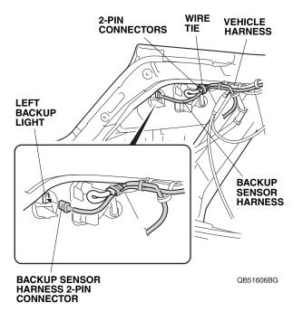
28. Secure the 2-pin connectors to the vehicle harness with one wire tie.
