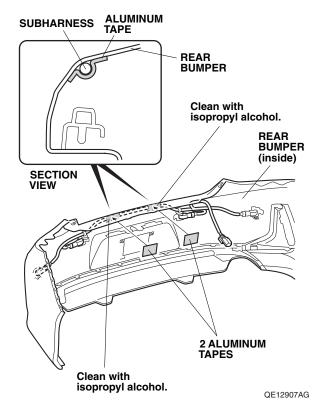
16. Secure the subharness to the rear bumper with two aluminum tapes.
