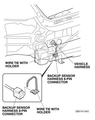
40. Install the connector clip on the backup sensor harness 8-pin connector, and secure it to the vehicle panel.
