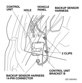
34. Secure the two clips on the backup sensor harness to the control unit bracket B and the hole in the vehicle panel.
