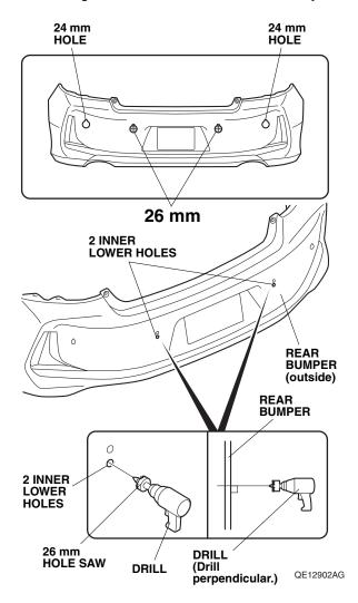
11. Using the sensor clips, install the left corner sensor into the 24 mm hole and the left center sensor into the 26 mm hole in the rear bumper. Note the direction and the pin location for each sensor.
