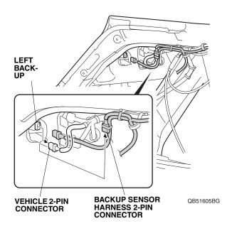
27. Plug the backup sensor harness 2-pin connector into the left backup light.
