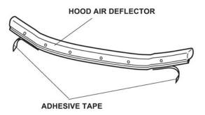
13. Align the holes on the hood air deflector with the brackets A, B, C. Install the hood air deflector with two screws, two collars, and four clips. Tighten the screws securely. Remove the adhesive backings.
