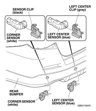
55. Secure the corner sensor (white) and left center sensor (blue) with sensor clip (black) and left center clip (gray) as shown.
