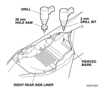
46. Insert the switch into the drilled hole, and install the switch bracket to the switch in the direction shown.
