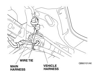
40. Reinstall the dummy connector to the main harness 4-pin connector.
