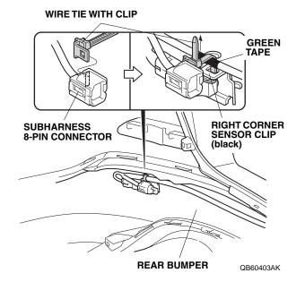
61. Using isopropyl alcohol on a shop towel, clean the areas where the aluminum tapes will attach. Secure the subharness to the rear bumper with four aluminum tapes.
