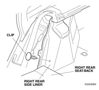
15. Remove the right cover (three clips and four tabs).
