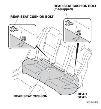
12. Pull out on the two knobs to release the two hooks, and remove the rear seat cushion.
