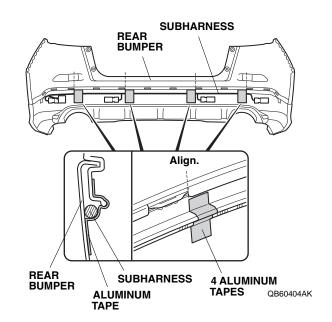
62. With the help of an assistant, bring the rear bumper to the vehicle, and plug the main harness 8-pin connector into the subharness 8-pin connector. Reinstall the rear bumper.
