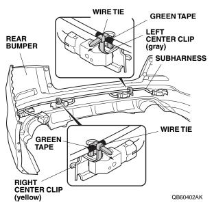
60. Secure the subharness 8-pin connector into the right corner sensor clip at green tape with one wire tie with clip.
