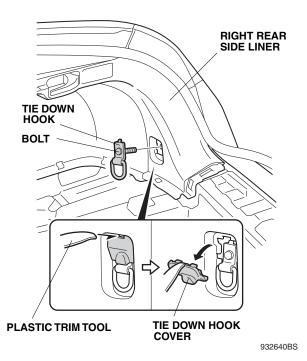
17. Using a plastic trim tool, remove the right side liner plastic cover. Remove the two screws under the cover.
