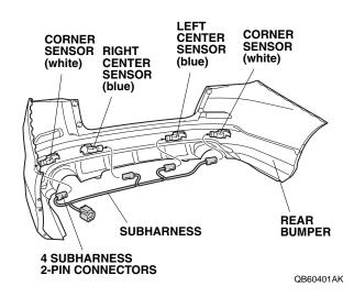
59. Secure the subharness into two center clips at two green tapes with the two wire ties.
