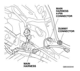
Route the main harness through the hole in the order shown. Set the main harness grommet into the vehicle panel.
