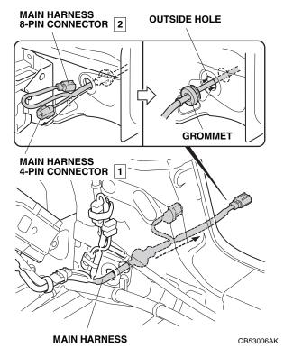
39. Secure the main harness to the vehicle harness with one wire tie.
