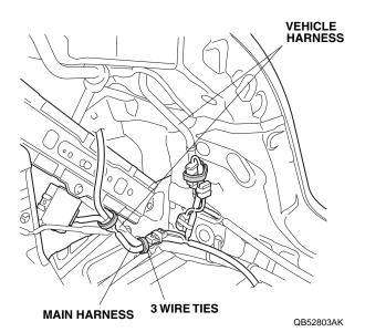
27. Using two wire ties, secure the main harness to the holes of the vehicle panel.
