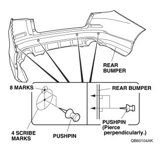
51. While wearing eye protection, drill the eight pierced marks with a 3 mm drill bit from the outside of the rear bumper.
