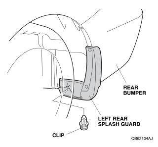
9. Repeat steps 5 through 8 to install the right rear splash guard on the right side of the vehicle.
