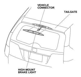
6. To keep metal shavings out of the tailgate, attach masking tape over the high-mount brake light opening.
