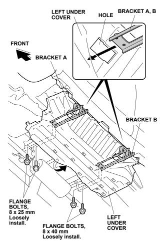
21. With the help of an assistant, bring the left under cover close to the vehicle and loosely install bracket A and bracket B to the vehicle panel using two 8 x 25 mm flange bolts and two 8 x 40 mm flange bolts. 22. Loosely install bracket C (FR) and bracket D (RR) to the vehicle panel using four 8 x 16 mm flange bolts.
