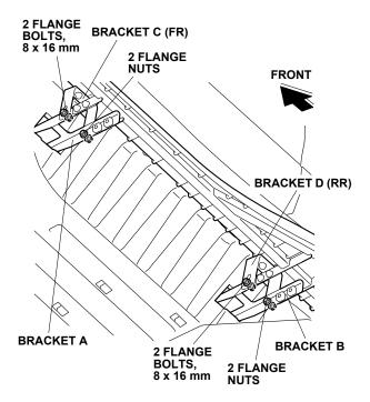
27. Torque the eight 8 x 16 mm flange bolts loosely installed in step 23 to 22 N·m (6 lbf·ft).
