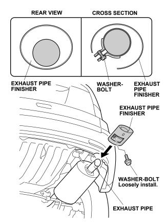
Continue to slide the exhaust pipe finisher in until it contacts the end of the exhaust pipe. While holding the exhaust pipe finisher firmly against the exhaust pipe, torque the washer bolt to 10 N·m (7 lbf·ft).
