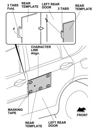
14. Align the rear template with the character line, and attach it to the left rear door using strips of masking tape.
