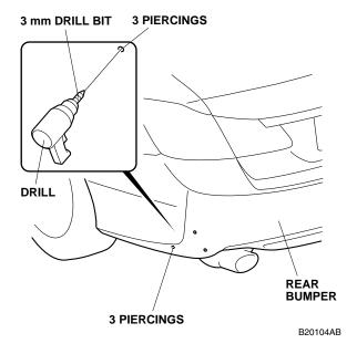
5. Enlarge the two upper holes to 12 mm using a 12 mm drill bit. Remove any burrs.
