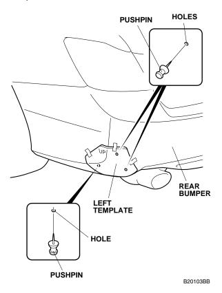
4. While wearing eye protection, drill the three piercings in the rear bumper with a 3 mm drill bit.
