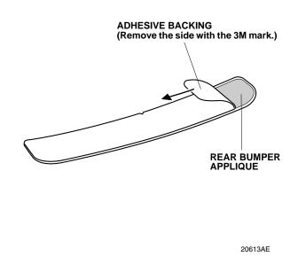
6. Spray the rear bumper applique with the 3M protective tape application solution.
