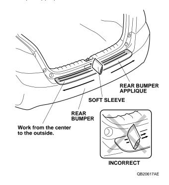
11. Slowly remove the protective film from the rear bumper applique. NOTE: Do not pull up on the protective film.
