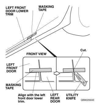
Using an utility knife, cut the masking tape along the gap of the left doors. Be careful not to damage the doors. 10. Peel back the adhesive backings, and tape them to the front surface of the left rear trim with masking tape. Remove the small the adhesive backings.
