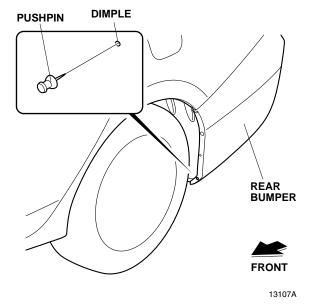
9. Pull away the rear bumper. Use a utility knife to cut the left rear inner fender in the area shown.
