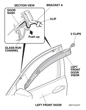
8. Secure the left front door visor to two brackets A with two clips. Make sure to push up on the brackets A while installing two clips.
