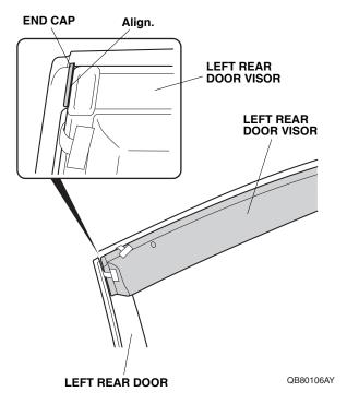
22. While applying light pressure against the left rear door visor, carefully remove the taped adhesive backings in the order shown. Make sure to push up on the brackets A while removing the adhesive backings.
