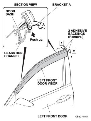
12. Using the palm of your hand, firmly press the left front door visor against the door sash.
