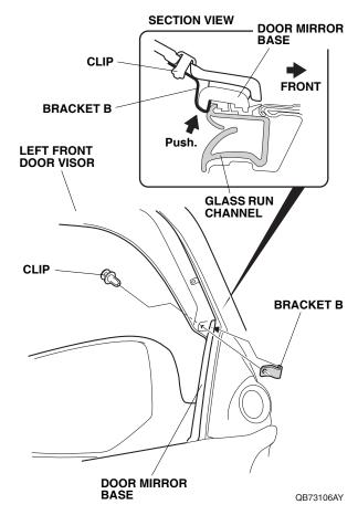
11. While applying light pressure against the left front door visor, carefully remove the taped adhesive backings in the order shown. Make sure to push up on the brackets A while removing the adhesive backings.
