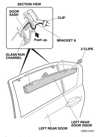
20. Secure the left rear door visor to two brackets A with two clips. Make sure to push up on the brackets A while installing two clips.
