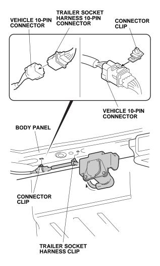
18. Install the connector clip into the vehicle 10-pin connector, and push the connector clip and trailer socket harness clip into the holes in the body panel.
