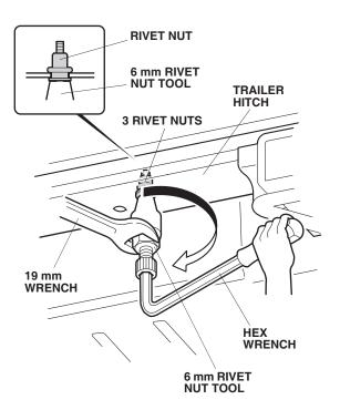
14. Remove the 6 mm rivet nut tool from the rivet nut by turning the hex wrench counterclockwise. Install rivet nuts into the two remaining holes in the trailer hitch.
