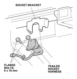
17. Plug the trailer socket harness 10-pin connector into the vehicle 10-pin connector.
