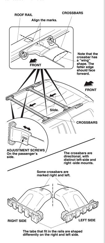
3. Tighten the eight thumbwheel screws to secure the crossbars to the roof rails.
