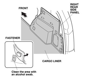
9. Align the holes on the cargo liner to the two tie-down hooks, anchor, and power outlet on the right rear side panel.
