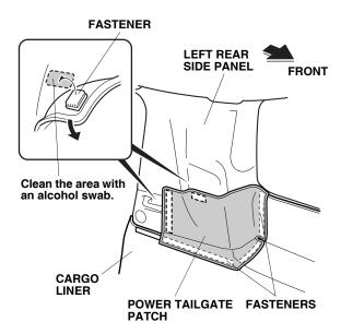
23. Align the power tailgate patch to the left rear side panel. Fold the power tailgate patch back and, using an alcohol swab, thoroughly clean the area where the fasteners will attach. After cleaning with the alcohol swabs, wait at least 3 minutes before continuing with the next step.
