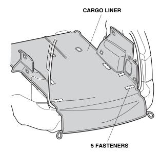
6. Attach five fasteners on the cargo liner to the cargo floor as shown.
