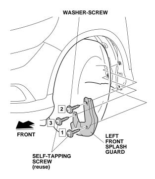
5. Turn the steering wheel fully clockwise, and repeat steps 2 through 4 to install the right front splash guard.
