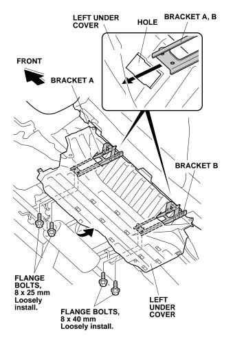
21. With the help of an assistant, bring the left under cover close to the vehicle and loosely install bracket A and bracket B to the vehicle panel using two 8 x 25 mm flange bolts and two 8 x 40 mm flange bolts.
