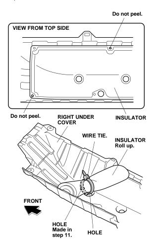
13. Align and attach the right front template and right rear template to the right under cover with masking tape in the areas shown.
