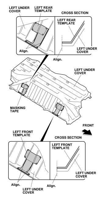
5. Using a pushpin, pierce the six marks on each templates.
