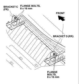
26. Torque the eight 8 x 16 mm flange bolts and eight flange nuts loosely installed in step 13 and 18 to 22 N·m (16 lbf·ft).
