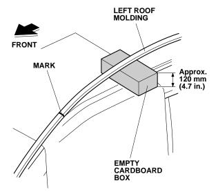
7. While wearing an eye protection, use an air saw to cut the left roof molding at the mark. Do not use a cutting wheel or shears to cut the left roof molding, it will damage the left roof molding. Have an assistant hold the rear edge while cutting.
