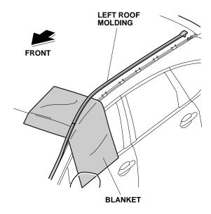
6. Place an empty cardboard box (approx. 120 mm tall) under the left roof molding near the mark.
