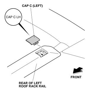
18. Repeat steps 1 through 17 to install the right roof rack rail on the right side of the vehicle.
