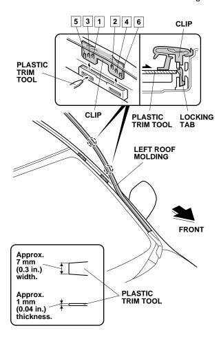
Place a blanket over the roof of vehicle under the left roof molding. Be careful not to deform the roof molding when measuring and cutting.
