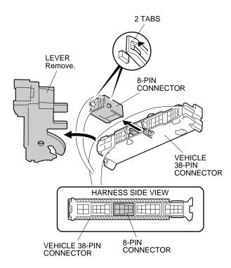
59. Remove the 8-pin connector from the vehicle 38-pin connector (two tabs).
