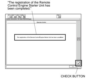
12. The following message will display: Check that the engine can be started by the Transmitter. Click on the check button.
