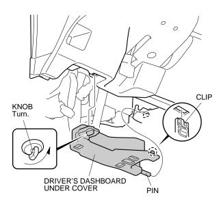
16. Remove the driver's dashboard lower cover (eight clips and unplug the vehicle connector).
