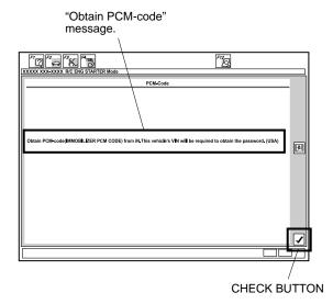
10. Input the PCM Code, then click the check button. NOTE: To ensure security, the PCM code (password) is changed everyday, so it is impossible to register the remote control engine starter if the dates of the PCM code acquisition and registration are different. The date of the HDS tester should also be the same.
