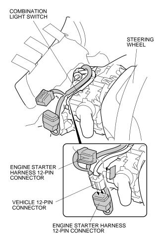
81. Plug the remaining engine starter harness 12-pin connector into the combination light switch.
