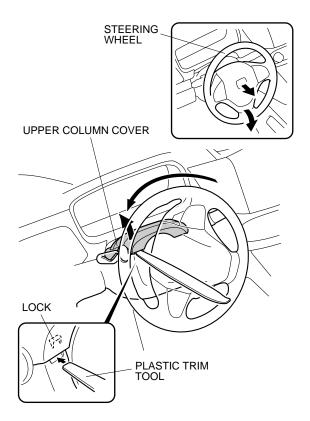
19. Using a plastic trim tool, release the lock as shown.
