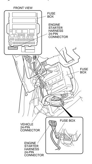
67. Secure the engine starter harness to the vehicle harness with two wire ties.
