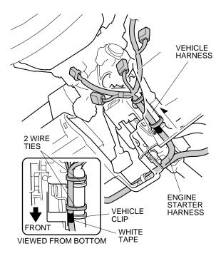
72. Align the white tape on the engine starter harness with the vehicle clip, and secure the engine starter harness to the vehicle harness with two wire ties as shown.
