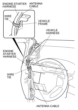
48. Secure the engine starter harness and the antenna cable to the vehicle harness with one wire tie.
