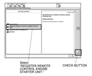
The following message will display: Obtain PCM code (IMMOBILIZER PCM CODE) from iN. This vehicle's VIN will be required to obtain the password (USA). Click on the check button.
