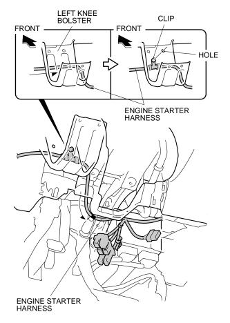
69. Secure the engine starter harness to the hole in the left knee bolster using the clip on the engine starter harness as shown.
