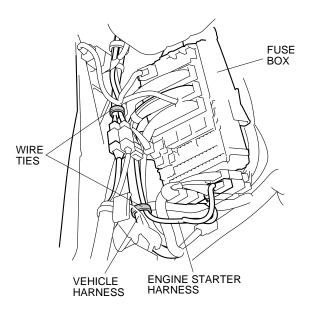
68. Route the engine starter harness under the dashboard and toward the steering wheel.
