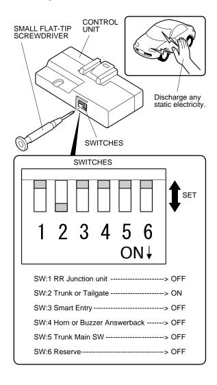
4. Using isopropyl alcohol on a shop towel, clean the control unit where the protective tape will attach. Remove the adhesive backing, and attach the protective tape to the control unit over the switches.
