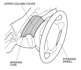
18. Lower the tilt lever, and turn the steering wheel 90° counterclockwise.
