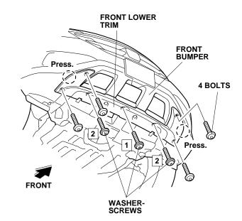
12. Install one bolt into each outboard 13 mm well nut and torque each bolt to 1.0 N·m (0.7 lbf·ft). Press the front lower trim against the front bumper when tightening the bolts on each side.
