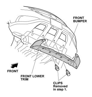
3. Using a pushpin, pierce the front bumper through the seven holes in the front lower trim.
