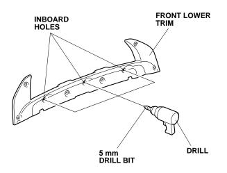
9. While wearing eye protection, drill the four outboard holes to 8 mm. First drill with a 5 mm drill bit, and finish with an 8 mm drill bit. Remove all burrs.
