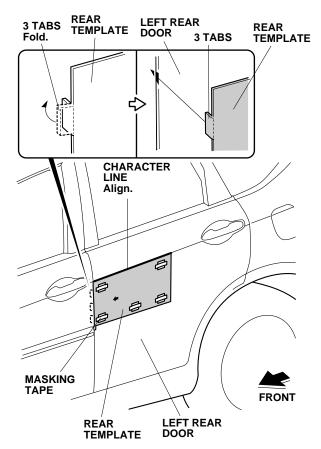
14. Align the rear template with the character line, and attach it to the left rear door using strips of masking tape.
