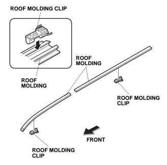
11. Reinstall the roof molding left cover.
