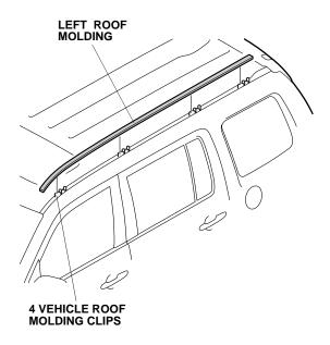
7. Remove and discard the four vehicle roof molding clips from the left roof molding or the stud bolt.
