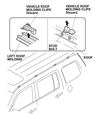
8. Remove any excess sealant from the stud bolts.
