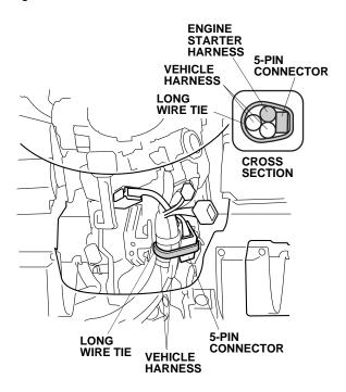
54. Unplug the vehicle 7-pin connector from the ignition switch, and plug the engine starter harness 7-pin connectors to the ignition switch and to the vehicle 7-pin connector.
