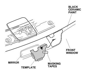
61. Using isopropyl alcohol on a shop towel, clean the area where the antenna will attach. Allow to dry before proceeding.
