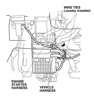
45. Route the engine starter harness 5-pin connector to the ignition switch.
