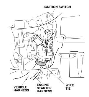
56. Adjust the steering wheel in, out, up, and down while you check the engine starter harness routing. If the harness is rubbing against the steering column bracket, check the installation and position of the wire ties installed in steps 53 and 55.
