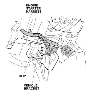
31. Route the engine starter harness relay block toward the right side of the vehicle.
