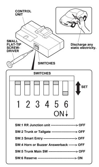
4. Check the settings of the switches on the control unit.
