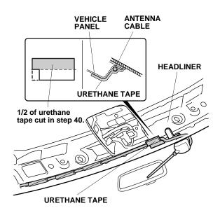
66. Clean the vehicle panel surface where the urethane tape will attach with isopropyl alcohol. Secure the antenna cable to the vehicle panel with the remaining part of the urethane tape you cut in step 40. Be careful not to crease the headliner.
