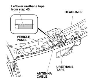
67. Route the antenna cable along the left A-pillar. Secure the antenna cable to the vehicle harness with four wire ties as shown.
