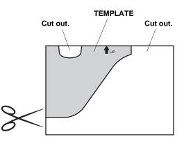
60. Align the template with edge of the black ceramic paint as shown, then secure the template to the windshield with masking tape.
