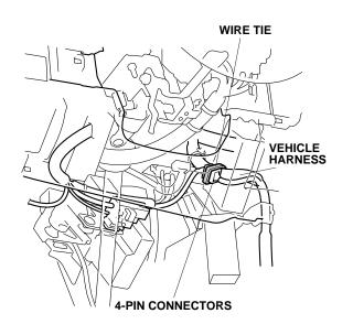
35. Align the green tape on the engine starter harness with the vehicle clip. Secure the engine starter harness to the vehicle harness with one wire tie.
