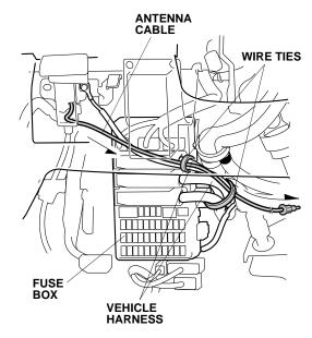
70. Route the antenna cable terminal toward the right side of the vehicle, and plug it into the control unit as shown.
