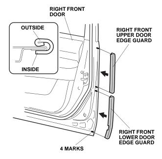
Make sure they are positioned correctly, then tap the right front door edge guards into position with a series of light taps with a rubber mallet. Once in place, do not remove, reposition, or reinstall the right front door edge guards or they will not hold securely.
