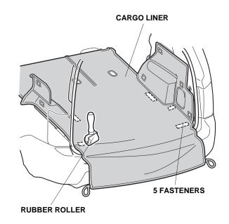
8. Align the cargo liner to the right rear side panel. Fold the cargo liner back and, using two alcohol swabs, thoroughly clean the area where the fasteners will attach. After cleaning with the alcohol swabs, wait at least 3 minutes before continuing to the next step.
