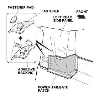
25. Remove the adhesive backing from two fastener pads, position the power tailgate patch, and attach the two fastener pads to the left rear side panel. Press the two fastener pads firmly against the side panel with the rubber roller. Go to step 30.
