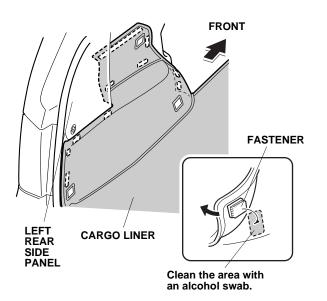
16. Align the holes on the cargo liner to the two tie-down hooks on the left rear side panel.
