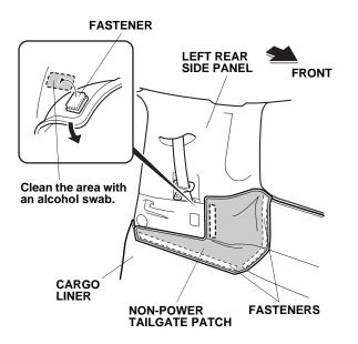
27. Align the non-power tailgate patch to the left rear side panel. Fold the non-power tailgate patch back and, using an alcohol swab, thoroughly clean the area where the fasteners will attach. After cleaning with the alcohol swab, wait at least 3 minutes before continuing with the next step.
