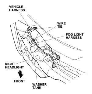
16. Continute routing the fog light harness under the right headlight as shown.
