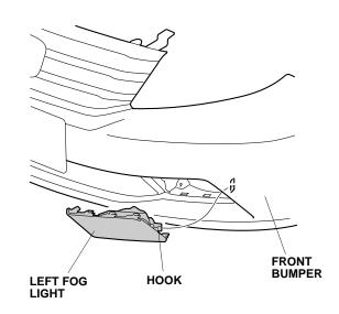
Secure the left fog light to the front bumper with one 5 x 16 mm washer-bolt.
