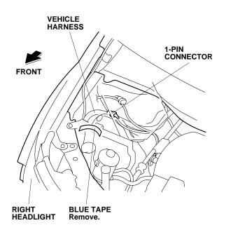
13. Plug the fog light harness 1-pin connector to the vehicle 1-pin connector.
