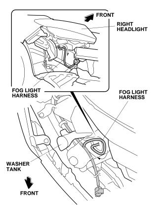
17. Install one wire tie with clip to the fog light harness at the green tape. Install the wire tie with clip into the vehicle panel hole.
