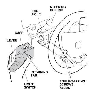
35. Install the new light switch to the steering column by pushing in on the case and setting the retaining tab into the tab hole. Do not push on the lever. Install the self-tapping screws removed in step 34.
