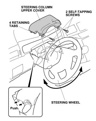
31. Remove the steering column upper cover (two self-tapping screws and four retaining tabs). Turn the steering wheel (right or left) to access each self-tapping screw.
