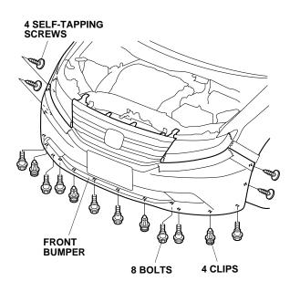
• Remove two top bolts from the front bumper. With the help of an assistant, remove the front bumper and set it on a blanket.
