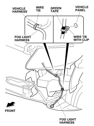
24. Secure the fog light harness to the vehicle harness with one wire tie.
