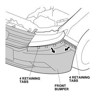
• Remove four self-tapping screws, eight bolts, and four clips from the front bumper.
