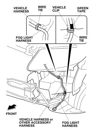
22. Secure the fog light harness to the vehicle harness with one wire tie. Go to step 25.
