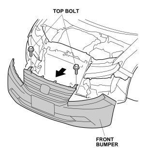
10. Remove the left front bumper trim cover (eight retaining tabs). Remove the right front bumper trim cover.
