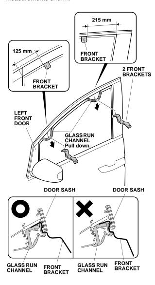
3. Reinstall the glass run channel to secure the two front brackets. Be sure the brackets are installed tightly to the door sash, and that the glass run channel is properly seated.
