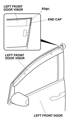
While applying light pressure against the left front door visor, carefully remove the adhesive backings.
