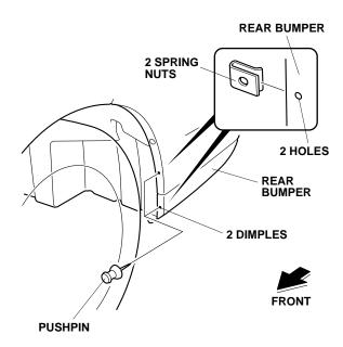
7. Install two spring nuts over the pierced holes in the rear bumper. Make sure the spring nuts are installed correctly.
